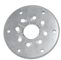
Grind the Star Cutter and Disc seen here to a 32 microfinish. Surfaces must be flat to within 0.001" T.I.R. Gap must be between 0.004" and 0.008" on these parts.
